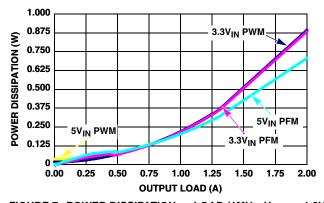
FIGURE 7. POWER DISSIPATION vs LOAD (1MHz,  $V_{OUT} = 1.8V$ )
