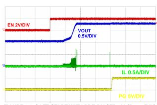
FIGURE 24. SOFT-START WITH PRE-BIASED 1V, (500µs/DIV)
