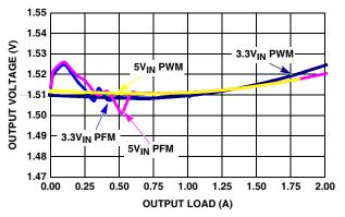
FIGURE 11. V<sub>OUT</sub> REGULATION vs LOAD (1MHz, V<sub>OUT</sub> = 1.5V)
