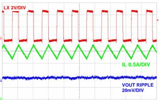
FIGURE 17. STEADY STATE OPERATION WITH FULL LOAD, (5μs/DIV)
