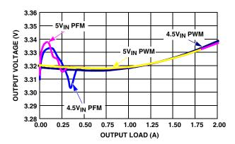
FIGURE 14.  $V_{OUT}$  REGULATION vs LOAD (1MHz,  $V_{OUT} = 3.3V$ )
