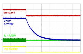
FIGURE 26. SOFT-DISCHARGE SHUTDOWN, (2ms/DIV)
