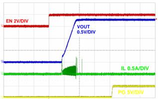
FIGURE 23. SOFT-START AT NO LOAD (PFM), (500µs/DIV)
