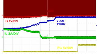
FIGURE 30. OUTPUT SHORT CIRCUIT RECOVERY, (500µs/DIV)
