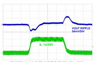
FIGURE 20. LOAD TRANSIENT (PWM), (50µs/DIV)
