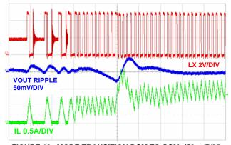
FIGURE 19. MODE TRANSITION DCM TO CCM, (50µs/DIV)
