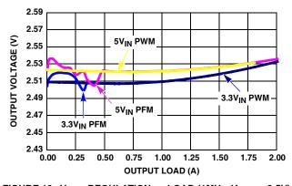
FIGURE 13.  $V_{OUT}$  REGULATION vs LOAD (1MHz,  $V_{OUT} = 2.5V$ )
