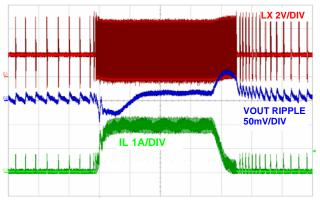
FIGURE 21. LOAD TRANSIENT (PFM), (500µs/DIV)
