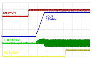
FIGURE 22. SOFT-START WITH NO LOAD (PWM), (500µs/DIV)
