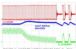
FIGURE 18. MODE TRANSITION CCM TO DCM, (5µs/DIV)
