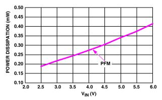
FIGURE 9. POWER DISSIPATION WITH NO LOAD vs  $V_{\mbox{\footnotesize{IN}}}$  (PFM  $V_{\mbox{\footnotesize{OUT}}}$  = 1.8V)
