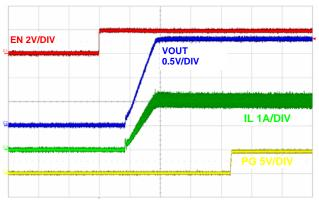
FIGURE 25. SOFT-START AT FULL LOAD, (2ms/DIV)
