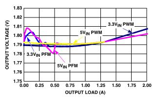
FIGURE 12. V<sub>OUT</sub> REGULATION vs LOAD (1MHz, V<sub>OUT</sub> = 1.8V)
