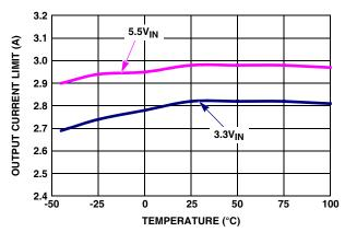
FIGURE 31. OUTPUT CURRENT LIMIT vs TEMPERATURE
